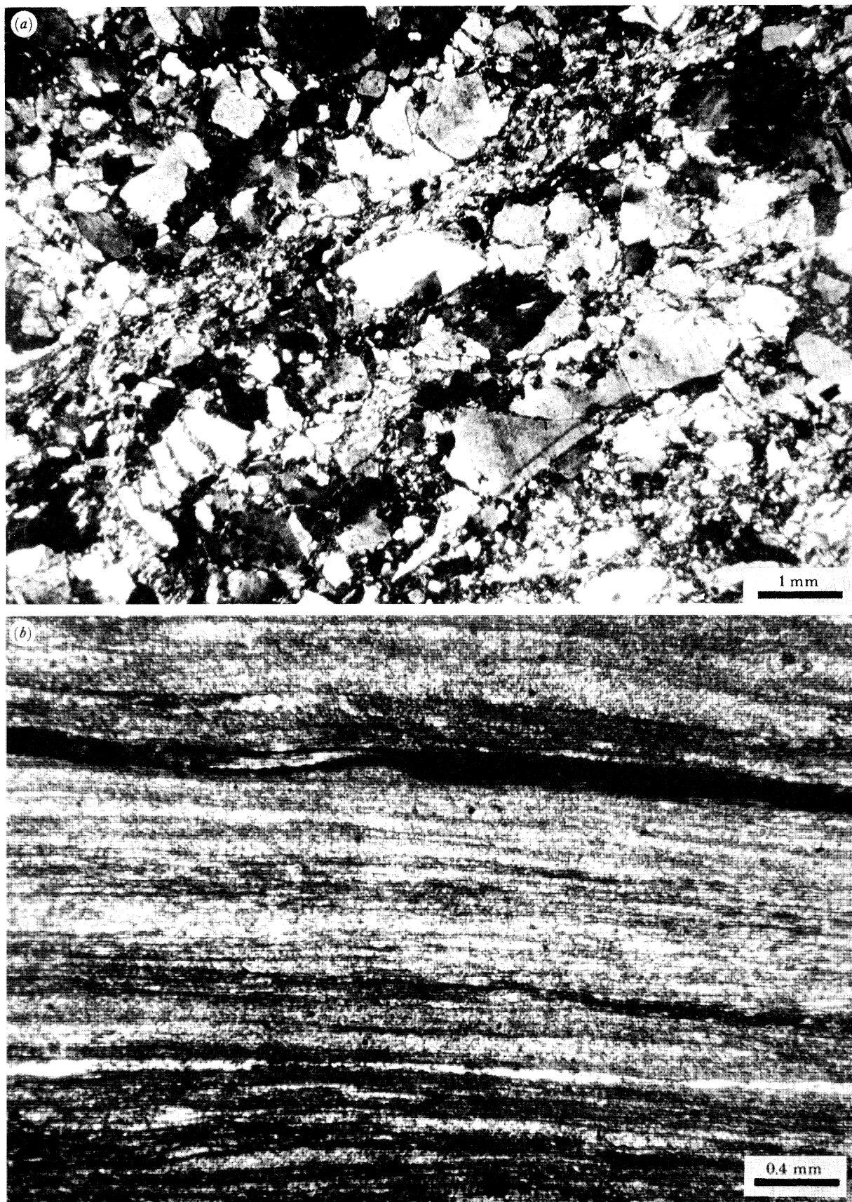
FIGURE 8. Microstructural changes associated with mylonite development in the Lewisian Gneiss along the Moine Thrust Zone, NW Scotland. Part A is the initial gneiss and part B is the quartz phyllosilicate mylonite (phylionite) arising from A at higher strains. (Bar scales: A = 1 mm, B = 0.4 mm.)
