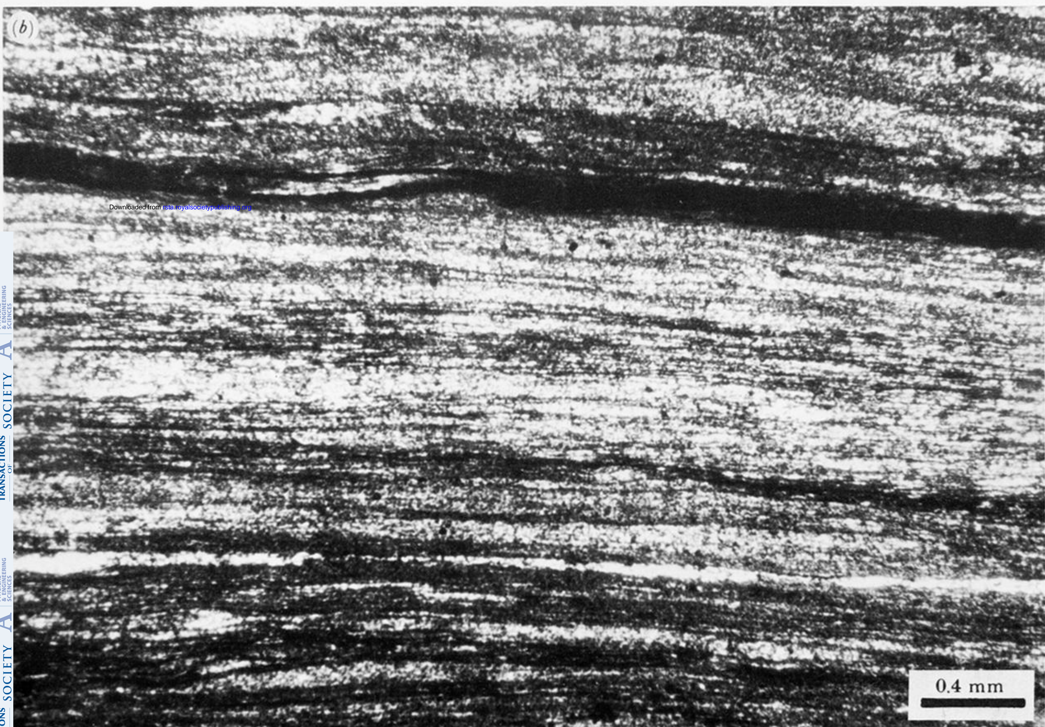
FIGURE 8. Microstructural changes associated with mylonite development in the Lewisian Gneiss along the Moine Thrust Zone, NW Scotland. Part A is the initial gneiss and part B is the quartz phyllosilicate mylonite (phylionite) arising from A at higher strains. (Bar scales: A = 1 mm, B = 0.4 mm.)
